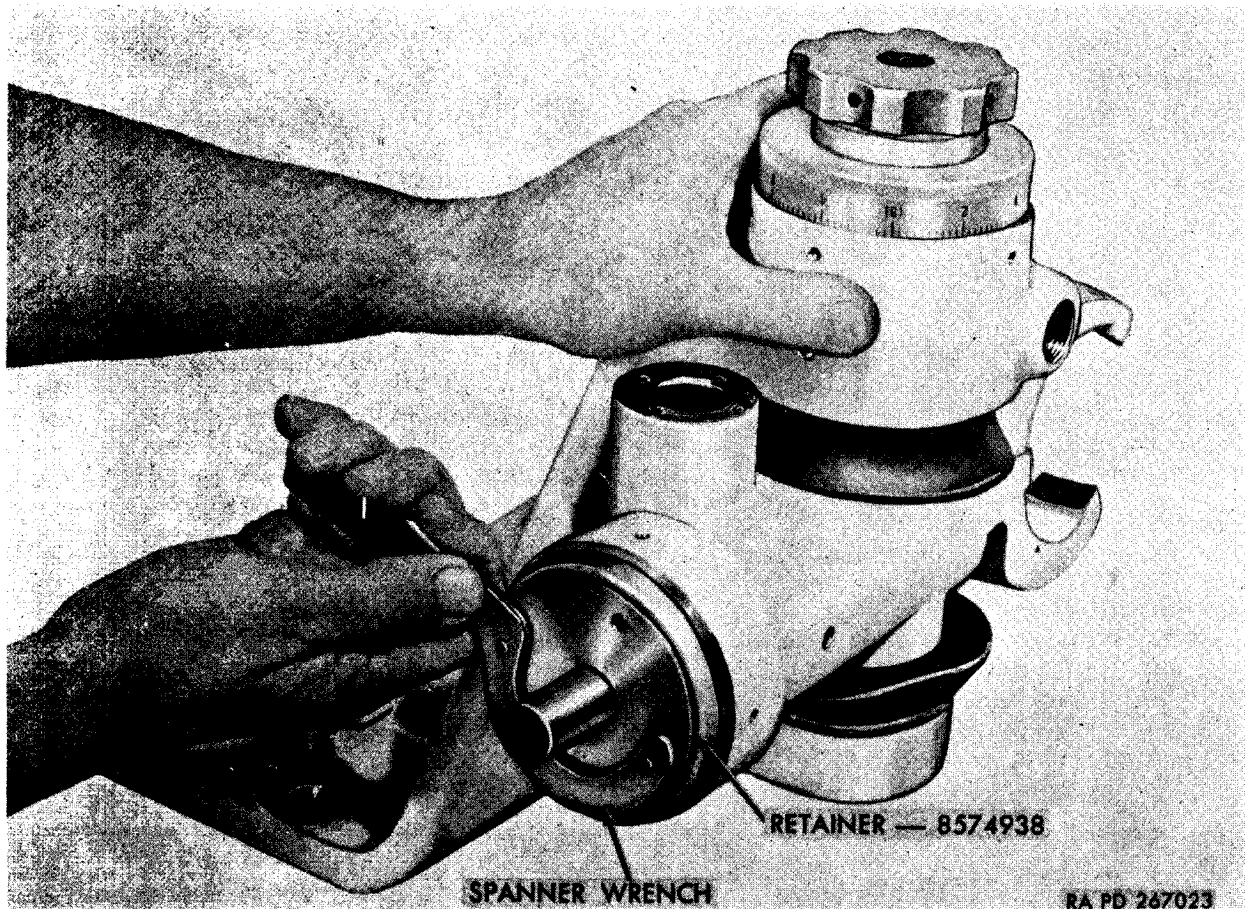
Figure 9. Removal or installation of retainer.
